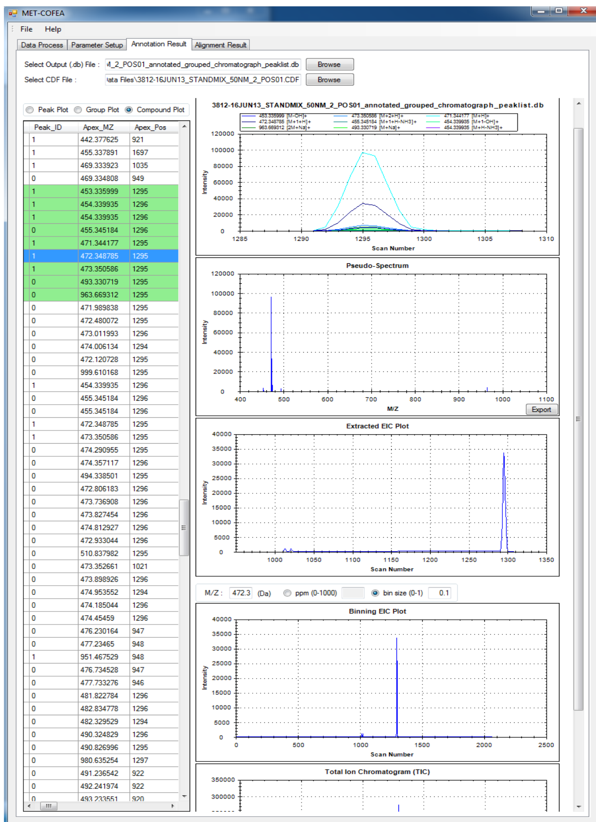
Fig.15 Visualization of the extracted EIC for the specific peak and the binning EIC from raw CDF file
